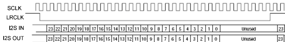
Figure 5 - Audio Data Timing Detail - I2S Mode, 64FS
